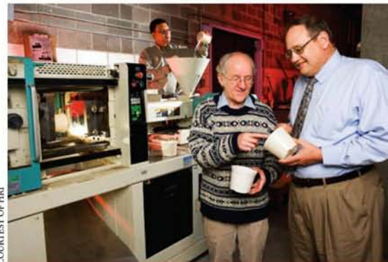
USDA-ARS chemist Walter Schmidt and HRI director of research Marc Tefteau examine plant containers made from chicken feathers.
